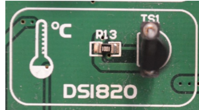
DS1820 temperature sensor connected. Make sure that the rounded side of the DS1820 matches the half circle on board
